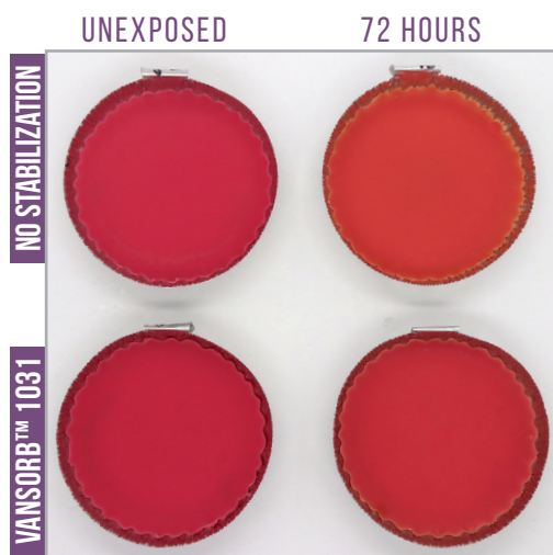
Soy wax candle formulation in a light box with continuing exposure to black light for 72 hours.
