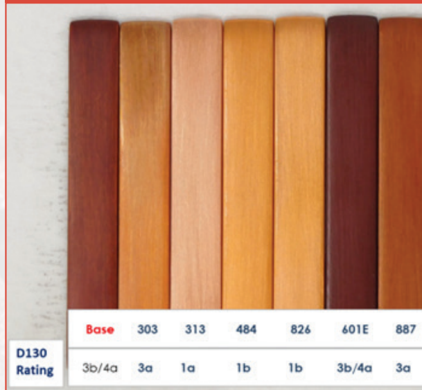
PICTURE 1: ASTM D130 RESULTS 24H @ 100 °C CORROSION TEST
