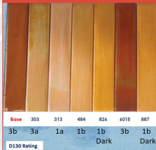
PICTURE 2: D130 RESULTS 3H @ 121 °C CORROSION TEST
